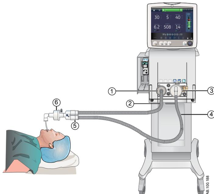
Figure 4-6 • Overview of setup and connections with a HME
