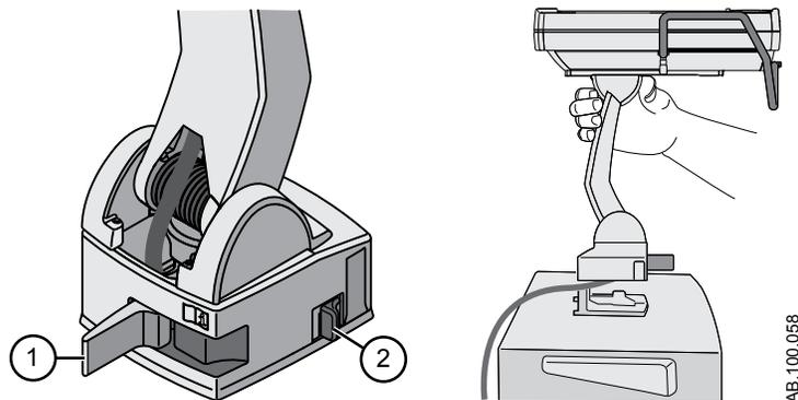
Figure 4-13 • Removing the display unit
