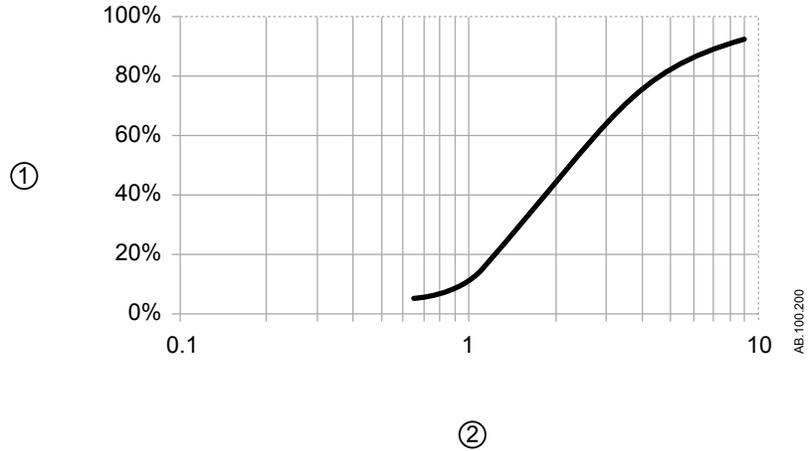
Figure 13-1 • Representative particle size distribution for Albuterol as per EN 13544-1 for use with the Aerogen Pro nebulizer
