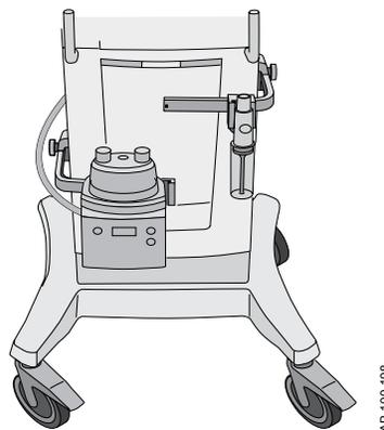
Figure 4-4 • Accessory rails shown with a water trap and a humidifier
