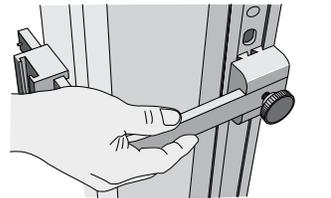
4. Tighten the thumbscrew to secure the rail at the desired height.
