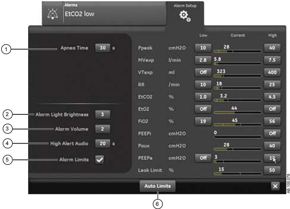
Figure 8-3 • Alarm setup menu
