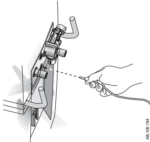
Figure 4-16 • Connecting the auxiliary pressure tubing
