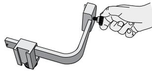
3. Use the leading edge of the wedge assembly to insert the rail into the dovetail located on either side of the ventilator cart.
