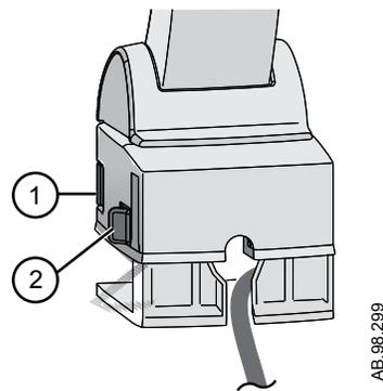
Figure 4-15 • Installing the display unit on the ventilator
