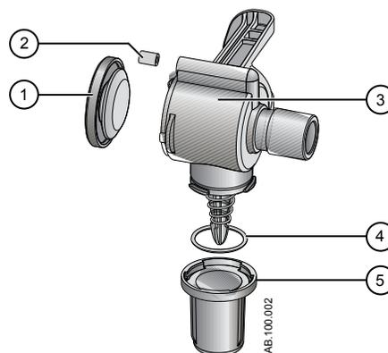
Figure 12-5 • Exhalation valve disassembly
