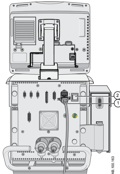
Figure 4-3 • Power connection and switch
