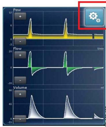
Figure 9-1 • Select the Settings icon to access waveform settings
