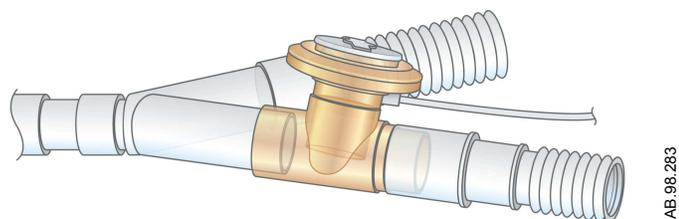
3. Attach the nebulizer cable to the nebulizer connection as shown, matching the red dots.
