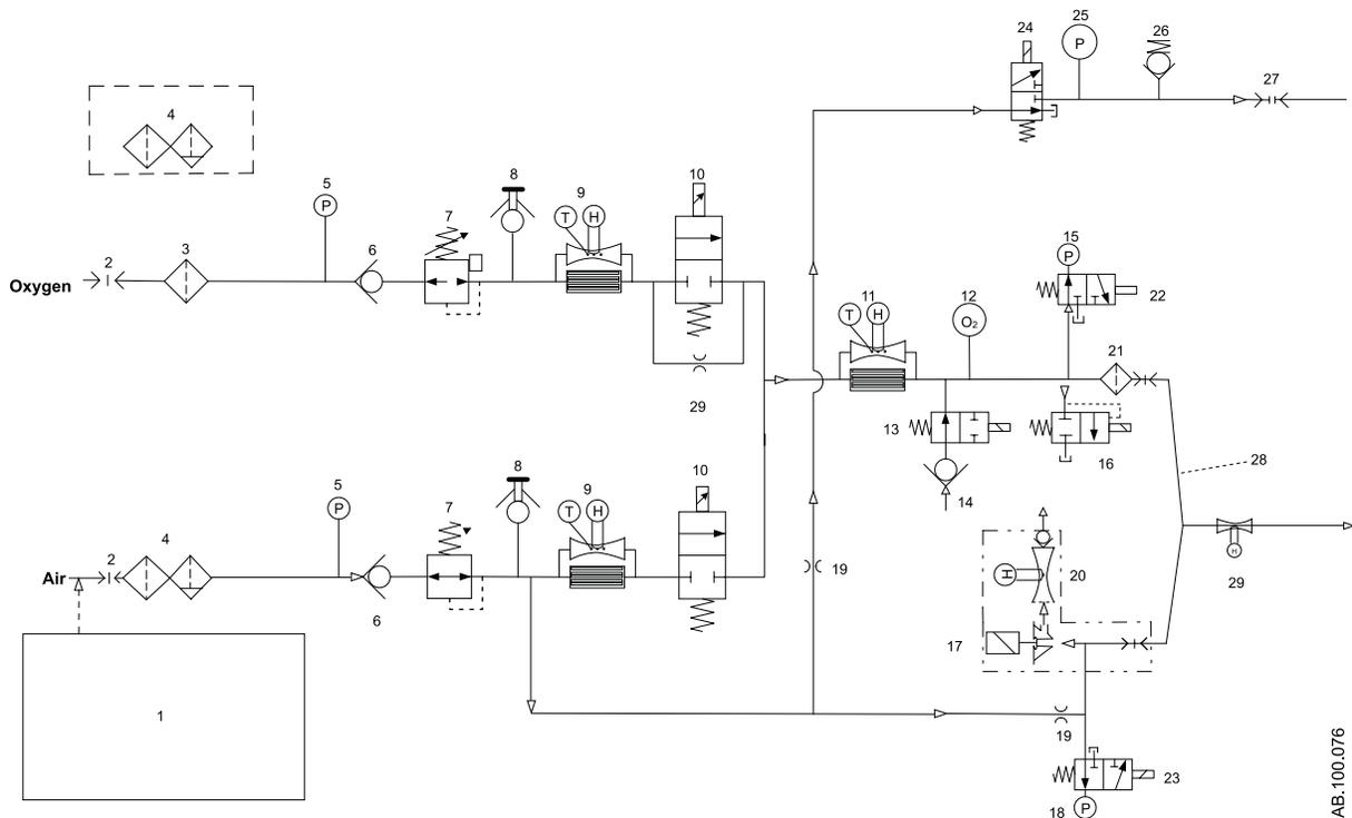
Figure 15-2 • Pneumatic architecture
