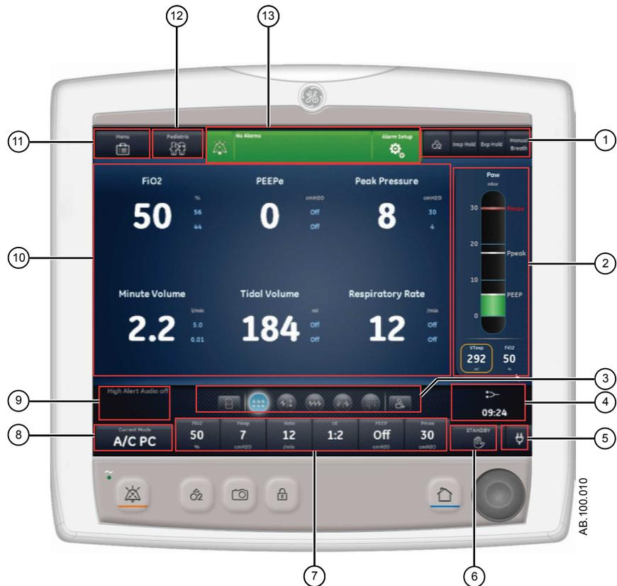
Figure 3-2 • Display user interface components
