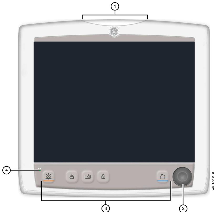
Figure 3-1 • Display controls and indicators
