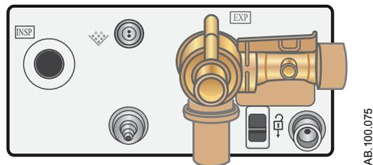
3. Unscrew the water trap to remove from the housing to empty or clean.
