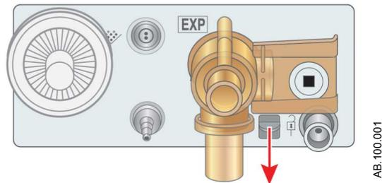
Figure 12-4 • Exhalation valve assembly
