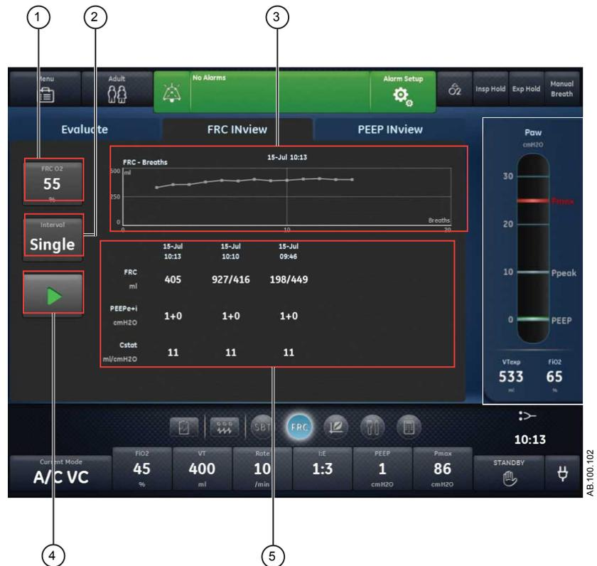
Figure 10-3 • FRC INview tab displaying three completed FRC measurements
