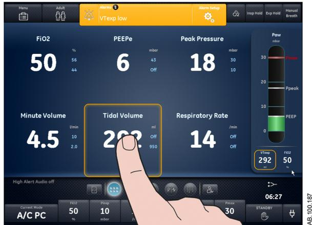
Figure 3-3 • Select inside of the border to open the Alarm Setup menu.
