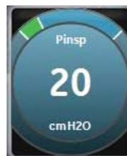
Figure 3-6 • The Trim Knob graphic is used to indicate that the use of the Trim Knob is necessary to change or confirm a setting
