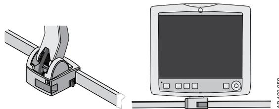
Figure 4-14 • Display unit mounted on a rail system
