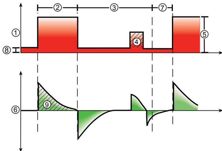
Figure 5-6 • SIMV PC waveforms
