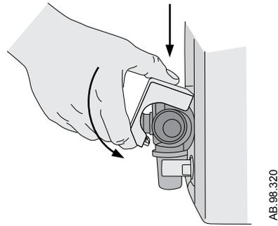
4. Align and match the red dots from the exhalation valve heater cable to the power cable and snap together.
