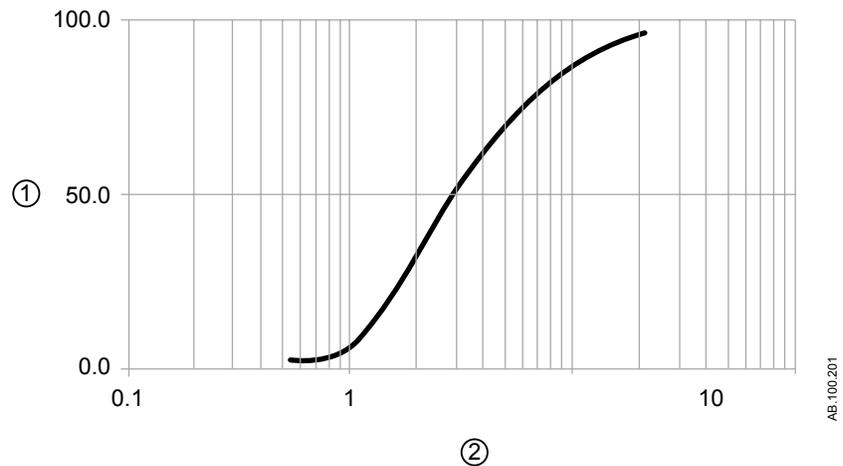
Figure 13-2 • Representative particle size distribution for Albuterol as per EN 13544-1 for use with the Aerogen Solo nebulizer
