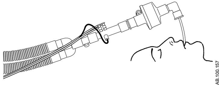
Figure 10-14 • D-Lite(+) sensor at 45° angle
