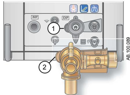
2. To remove the housing, press down on the latch to release the exhalation valve housing and then pull the housing from the ventilator.
