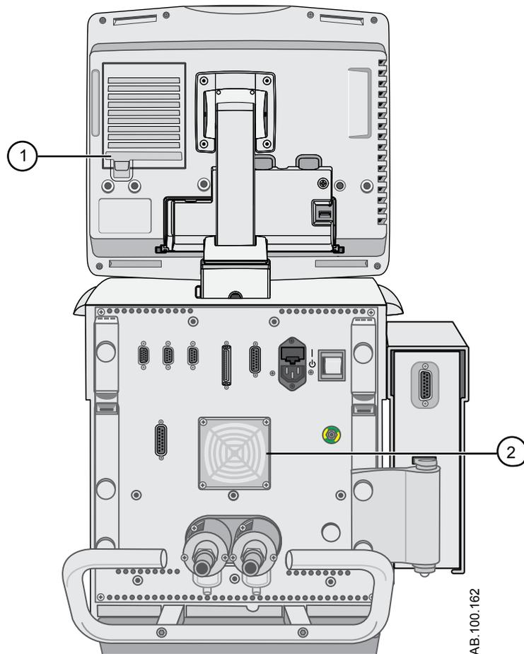
Figure 12-1 • Display and ventilator housing fan filters
