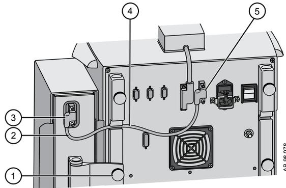
Figure 4-10 • Attaching and connecting the airway module bay
