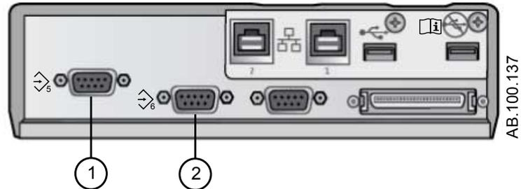
Figure 4-19 • Communication Port 5 (1) and Port 6 (2)
