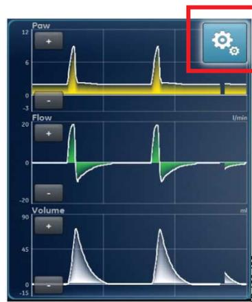
Figure 23-1 • Select the Settings icon to access waveform settings
