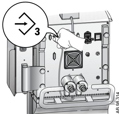
2. Thread the cable through the rear channel to the front of the ventilator.
