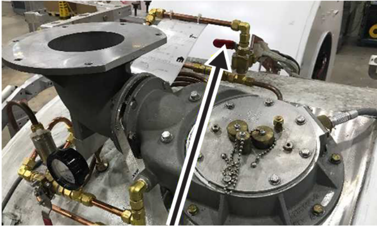
Figure 3-12 V3 valve in the closed position
