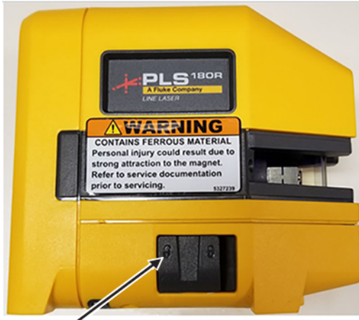
Figure 7-15 Laser level in self-leveling mode (unlocked position)
