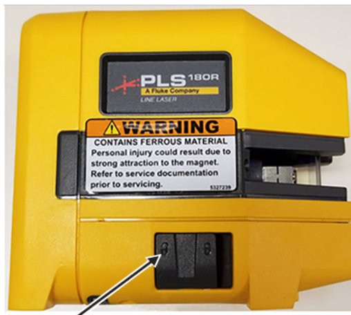
Figure 5-9 Laser level in self-leveling mode (unlocked position)
