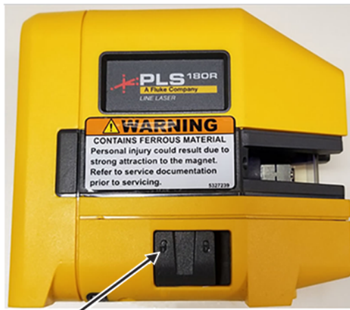
Figure 5-12 Laser level in self-leveling mode (unlocked position)
