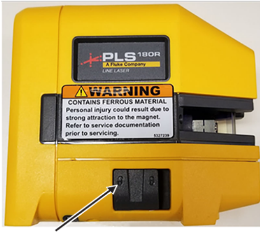
Figure 6-16 Laser level in self-leveling mode (unlocked position)
