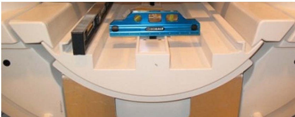
Figure 6-17 Magnet leveling, left-to-right
