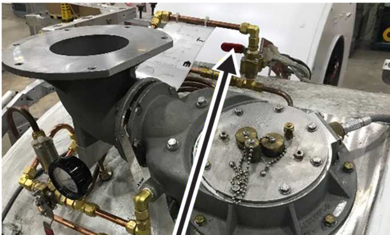
Figure 3-10 V3 valve in the closed position
