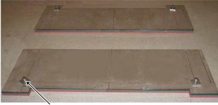
Figure 7-3 Surface mounted vibroacoustic damping mats
