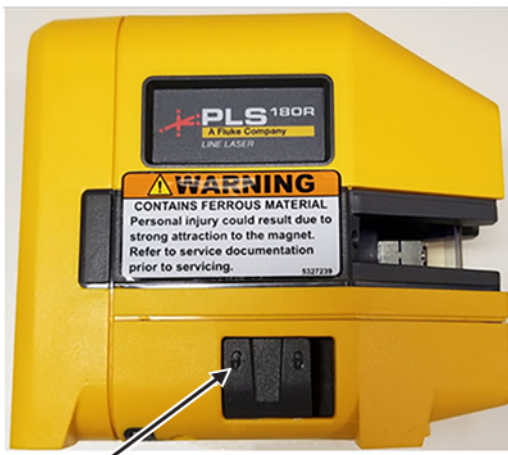
Figure 5-8 Laser level in self-leveling mode (unlocked position)
