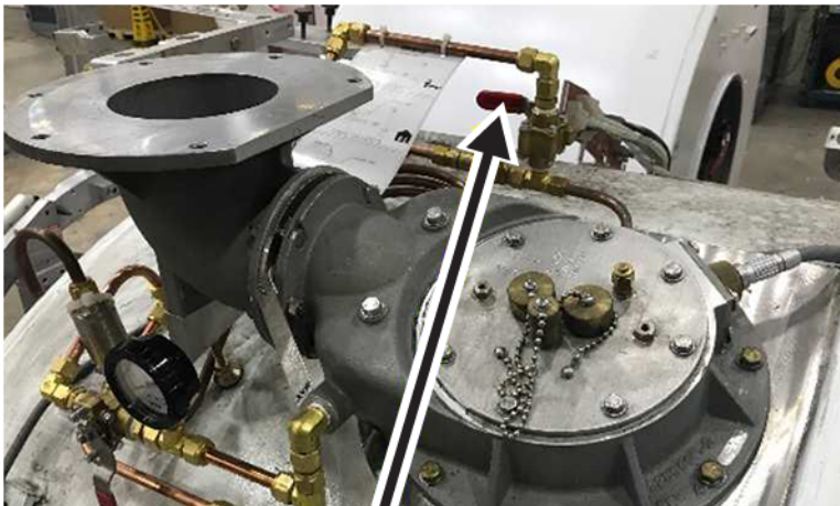
Figure 3-12 V3 valve in the closed position
