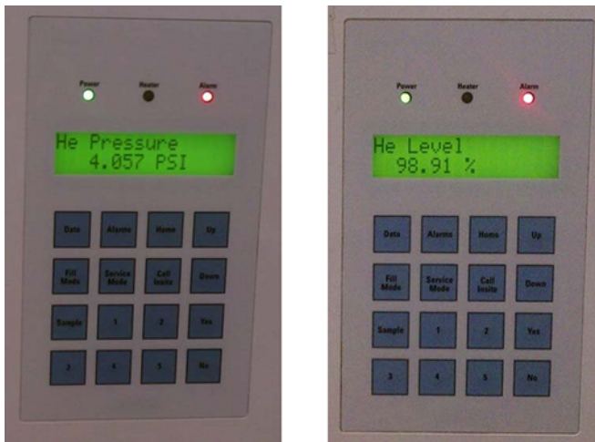
Figure 3-13 Magnet Monitor front panel user interface, He Pressure (psig) (left) and He Level (%) (right)
