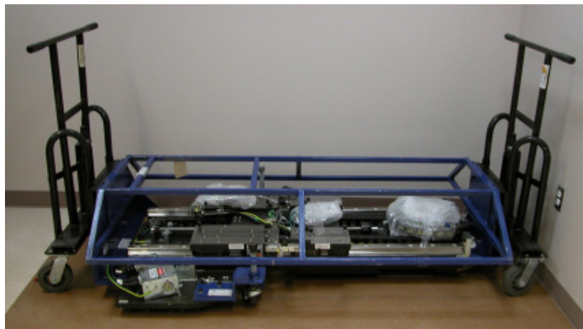
Illustration 1-2: PET Base and Retractor Assembly, with Shipping Dollies
