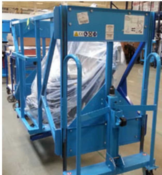
Illustration 1-4: PET Source Ring and Trailer, with Shipping Dollies and Side Rails
