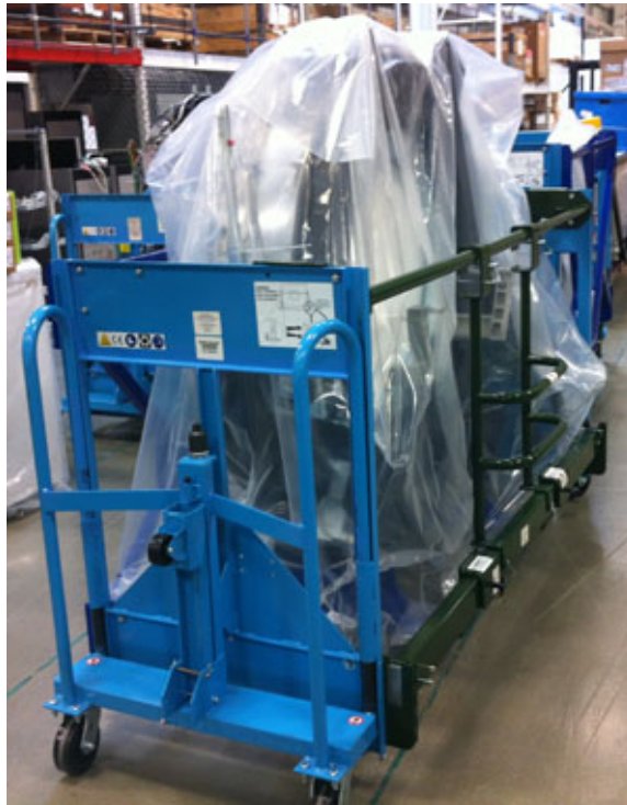
Illustration 1-4: PET Source Ring and Trailer, with Shipping Dollies and Side Rails
