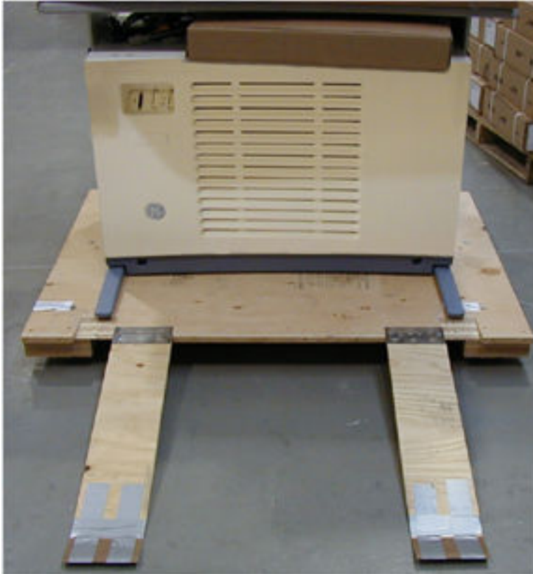
Figure 14-2 Console on skid with ramps exposed for unloading
